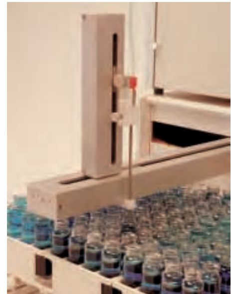
It is a fully unattended, self-regulating laboratory system that has been designed to seamlessly integrate into a company's operating practices. It adjusts to actual test fluid conditions and overall lab constraints, can measure viscosity from virtually any sample vial, and can deliver results to any information management system.
